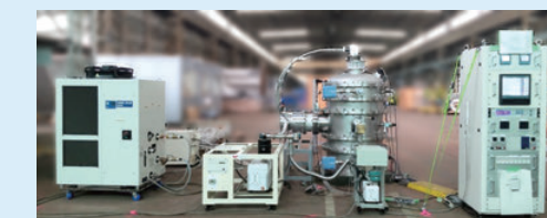
Vacuum exhaust prototype for liquefied hydrogen storage tank
