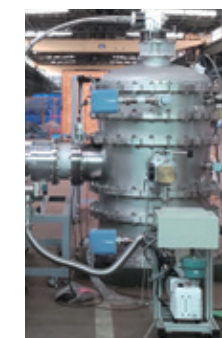
Vacuum insulation testing equipment
