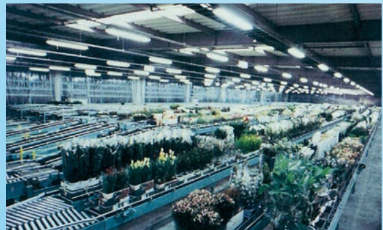
World's first conveyor-based automatic handling system for a potted plant market
